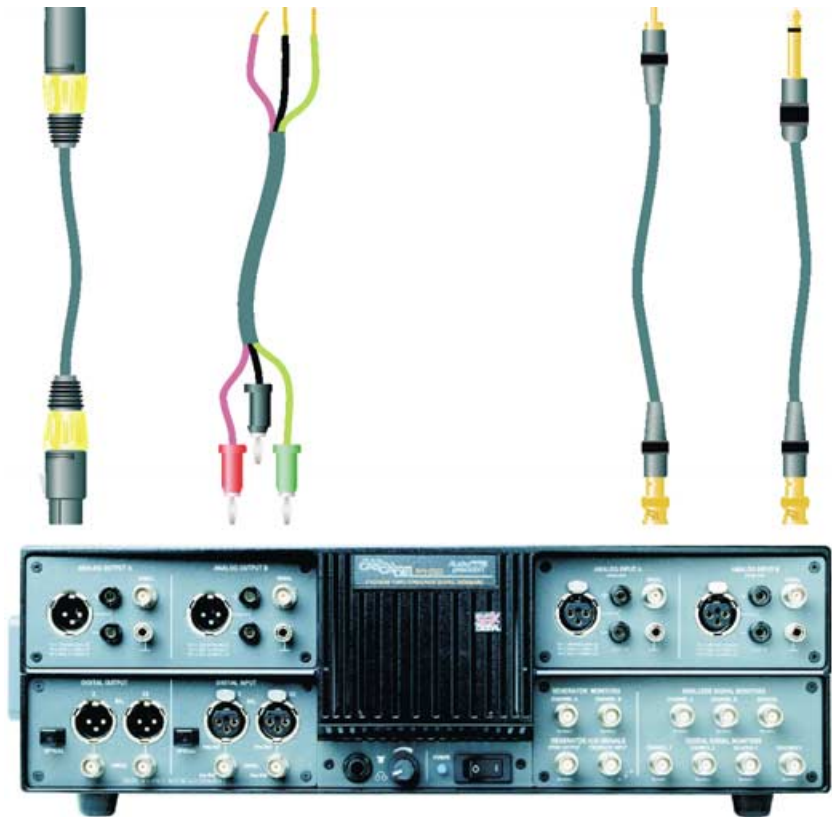
Figure 5-3. Typical balanced and unbalanced connections
